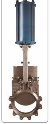
Our entire knife gate has a solid one-piece cast body with integrally cast gate jams and guides. They are full port and designed with blow out proof packing glands and nylock locking nuts. Our valves are designed and tested to Tappi TIS 405-8 and MSS-SP81 standards; our full lug pattern flanges conform to ASME B16.5.
